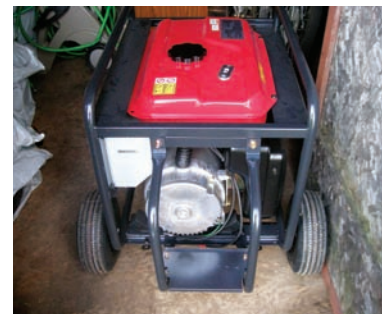
Emergency generators can provide backup power for sump-pumps and other household electric appliances during power outages.
