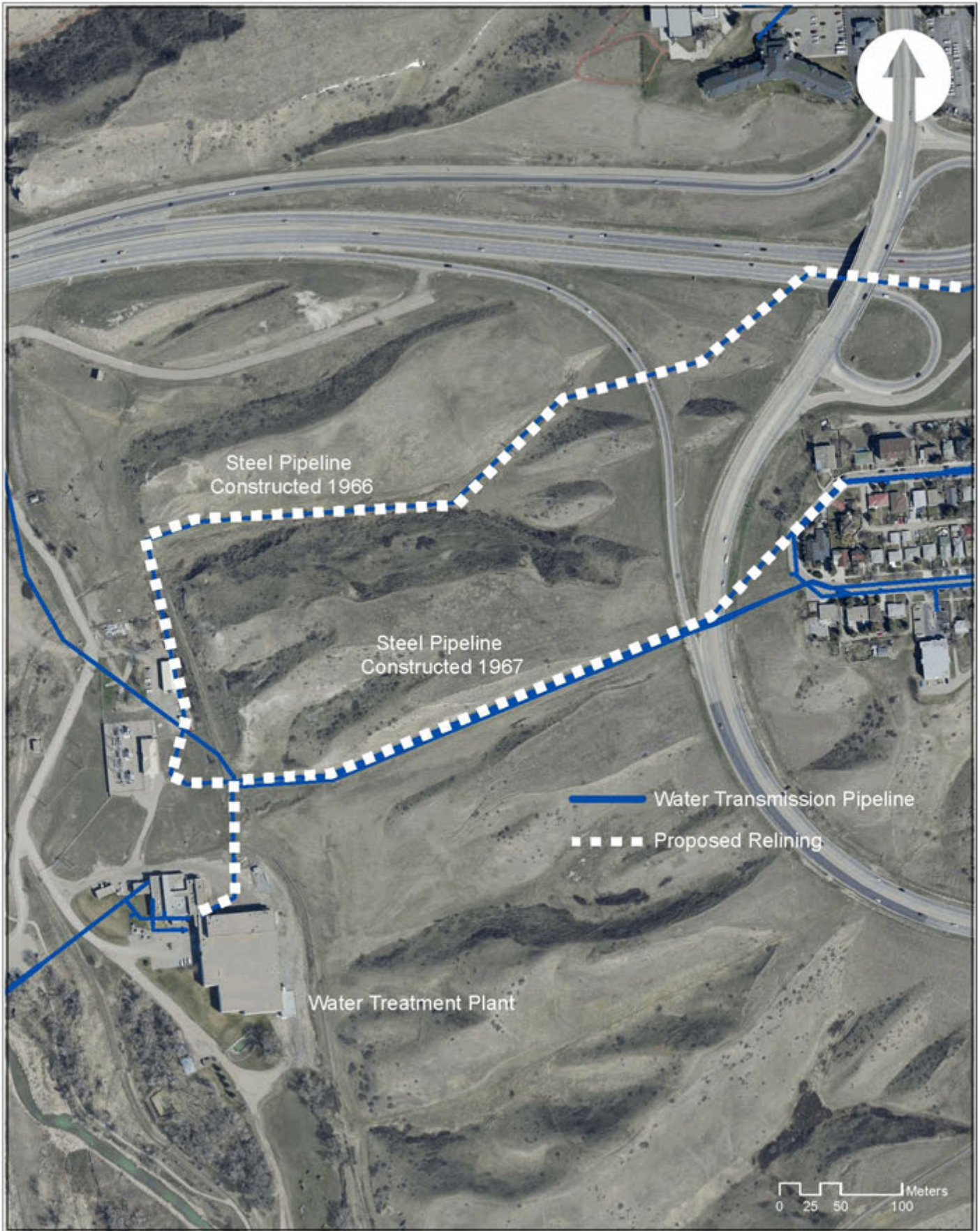
Water Treatment Plant Transmission Pipeline Rehabilitation
