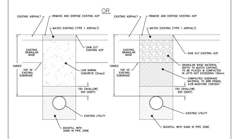
NOTE: LOW SHRINK CONCRETE 2mpa - SLUMP 75-125mm
