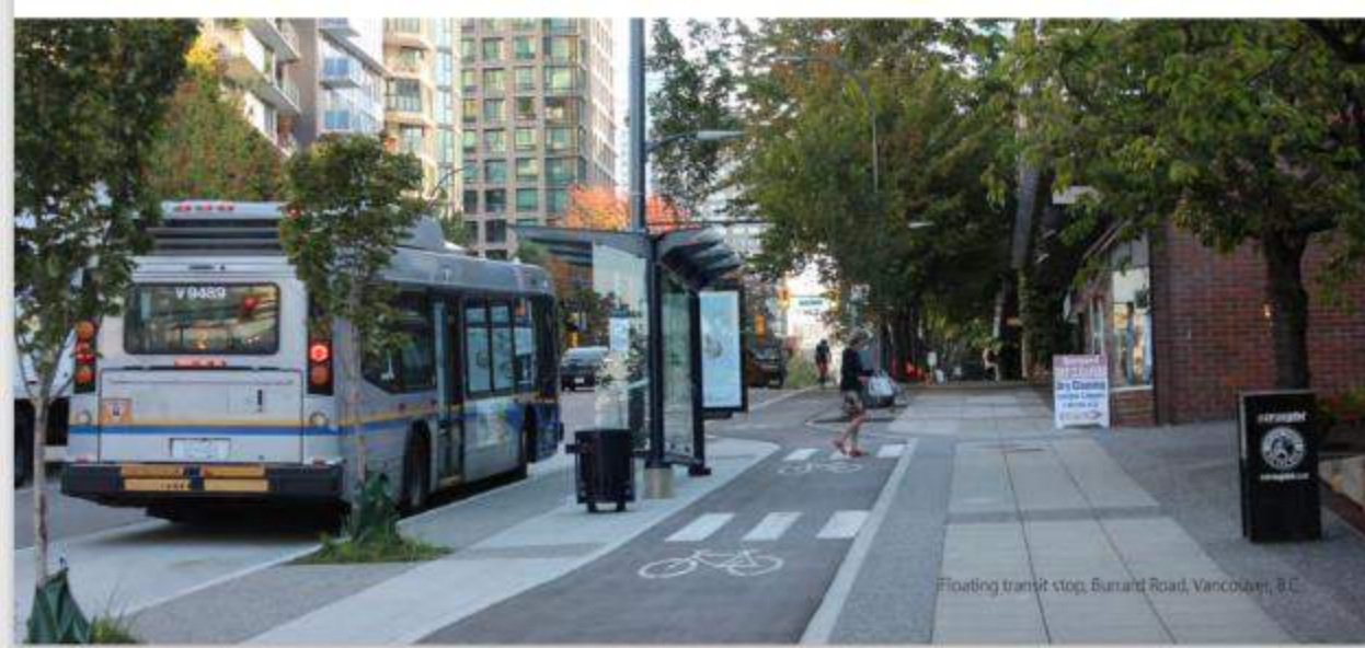
Figure 9-11: Example Floating Transit Stop (Burrard Street Vancouver, BC) Source: Page H-12, BC Active Transportation Design Guide
