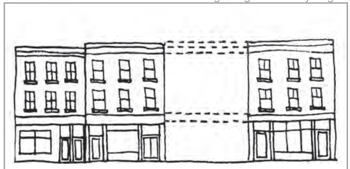
Consistent horizontal alignment of façade elements
