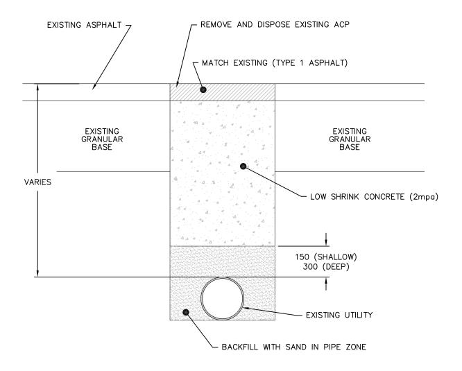
NOTE: LOW SHRINK CONCRETE 2mpa - SLUMP 75-125mm
