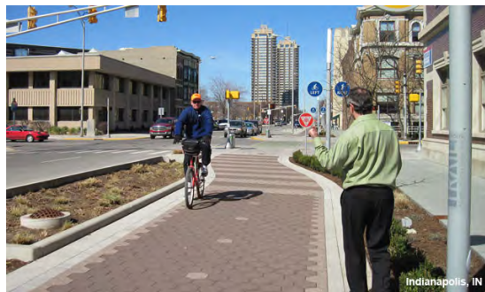
An example of a cycle track at a roadway intersection. Cycle tracks physically separate bicycles from vehicular traffic, increasing the comfort level of bicyclists Source: National Assoc. of City Transportation Officials “ http://nacto.org/cities-for-cycling/design-guide/cycle-tracks/ ”
