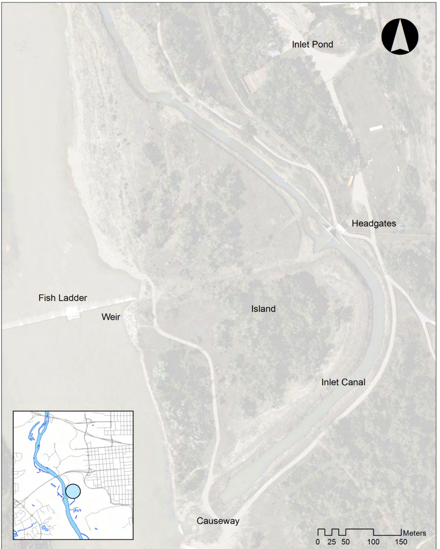
Water Treatment Plant River Intake Conceptual Design
